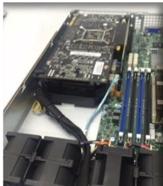
Ultrakompakt: 1 active-cooled Dual-Slot GTX-GPU in 1U...
